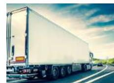
Trailer made with lightweight composite panels
